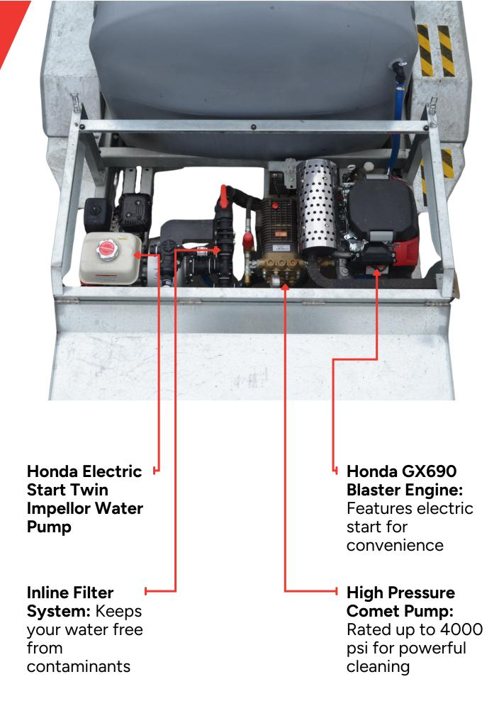
Purpose Built Trailer: Designed specifically for optimal performance and durability
